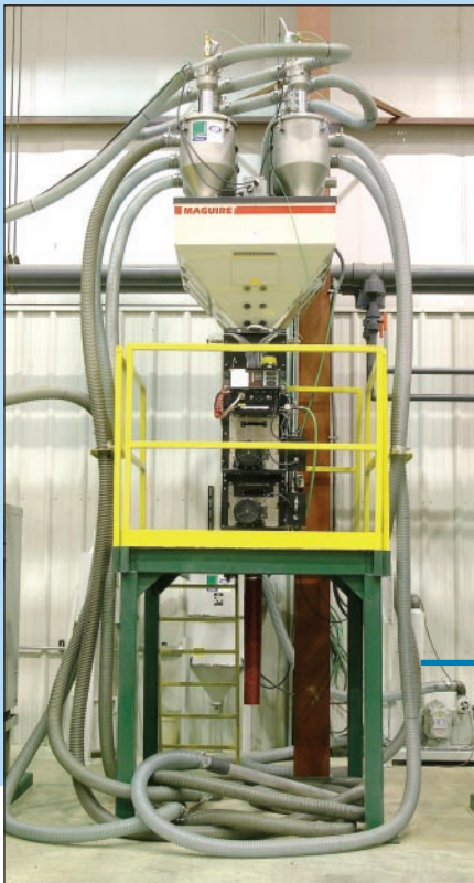
Up to six material components can be blended at the press using these weigh scale blenders.
